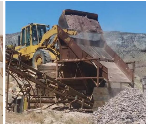
Preparing fluorspar for sorting
